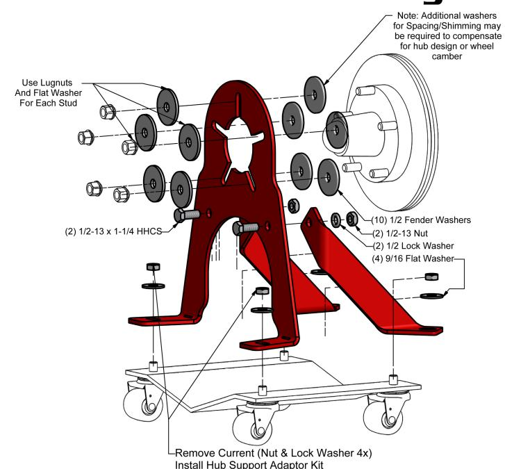
Reinstall Nuts And Washers Provided With Kit (As Shown) NOTE: Install all bolts loosely, and tighten sequentially
