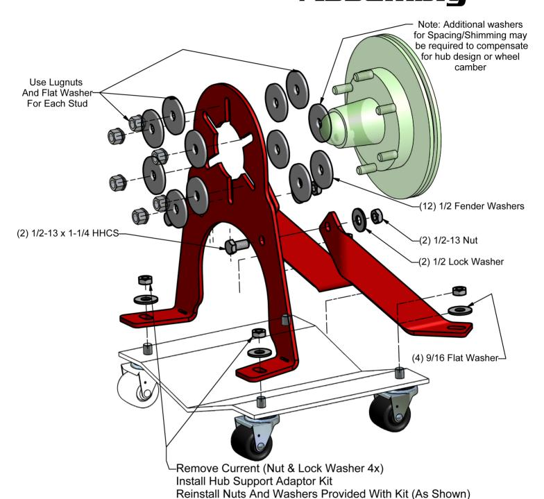
NOTE: Install all bolts loosely, and tighten sequentially until all bolts are tight. Do not over-tighten, see note below.
